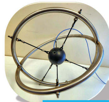
Marine acoustic particle motion sensor prototype, developed on partnership with Seiche Marine Acoustic Solutions
